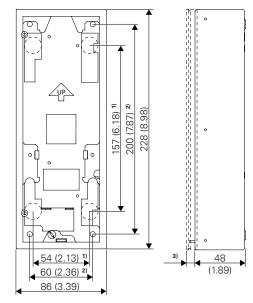
$^{1)}$  Dimensions for cable feed-through (ø 14 mm/0.55 in)  $^{2)}$  Dimensions for mounting holes (ø 5 mm/0.2 in)
